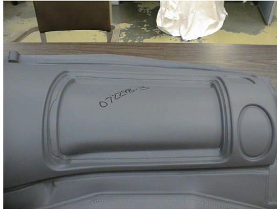
**Figure 2. Typical dashboard airbag release panel**
