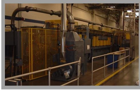
**Figure 3. Controlled Atmospheric Braze (CAB) furnace**
