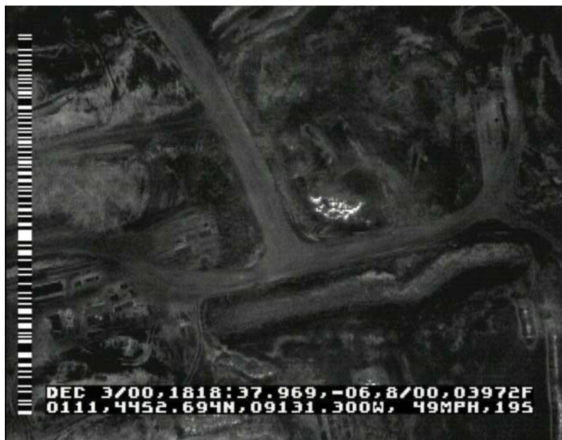
Figure 5. Thermograph of a subsurface landfill fire.
