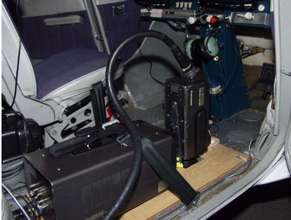
Figure 1. Photograph of a large format infrared imager, fixed-mounted in a light aircraft.
