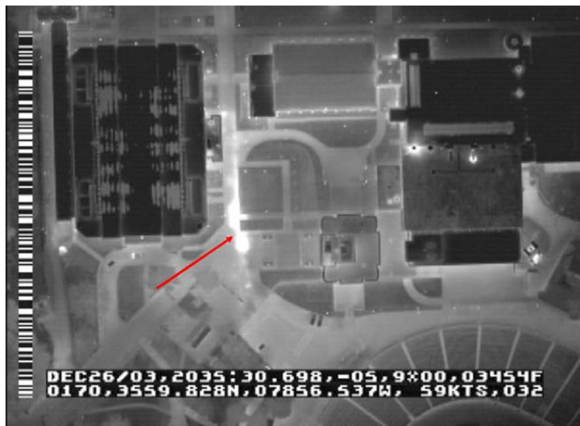
Figure 4. Thermograph of an underground steam system leak.
