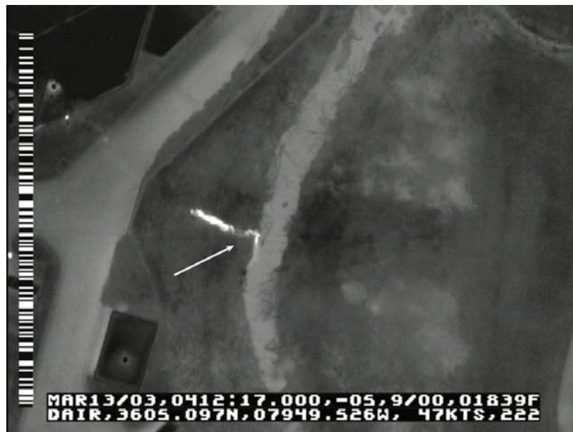
Figure 3. Thermograph of a stormwater drainage system outfall flowing into a creek.
