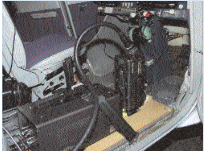
Figure 1. Whether using a helicopter or an airplane, your thermographer needs a fixed-mounted large-format infrared imager.
