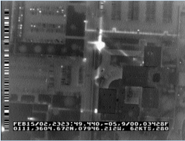
Figure 6. This infrared image shows a leak in a university steam system slightly above the center of the image.
