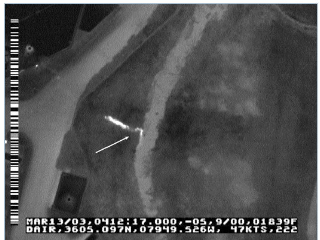
Figure 4. With infrared thermography, thermographers can see where liquids run into streams, lakes, and rivers. Here is stormwater drainage system flowing into a creek.
