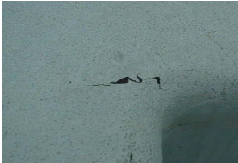
Figure 1. Photograph of a defect on the port side cockpit on US49
