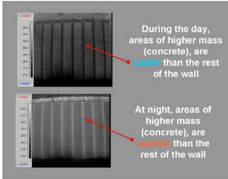
Figure 5. Thermograms showing daytime and nighttime temperature patterns.
