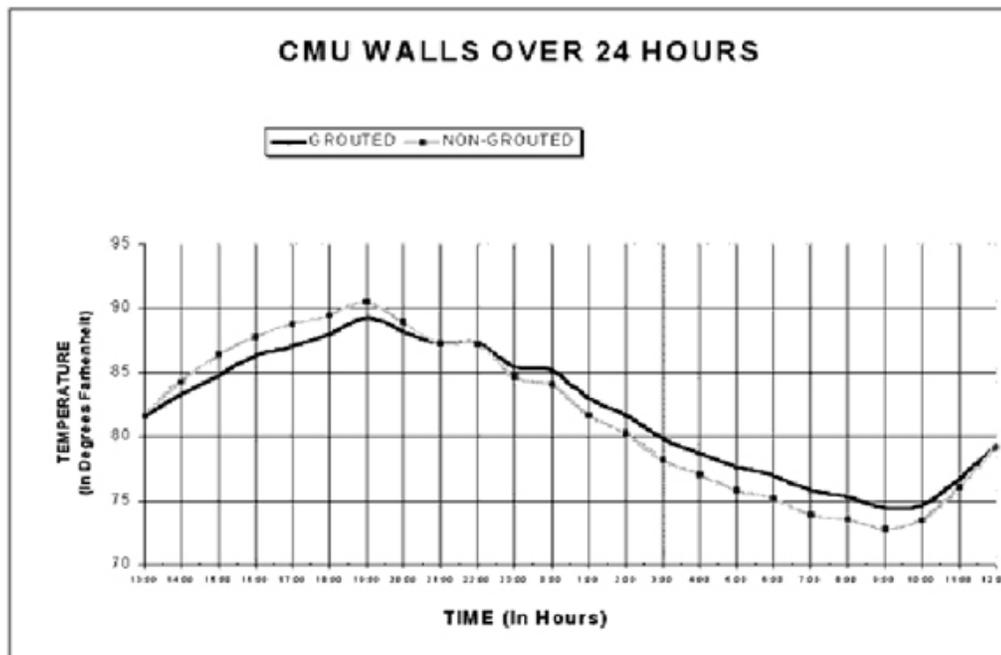
Fig. 6 Time vs. temperature plot of a South-facing CMU wall, over a 24-hour period.
