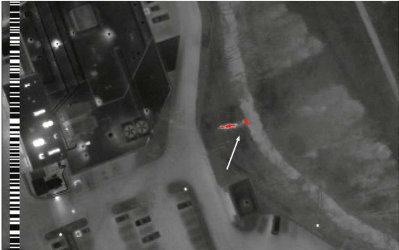
Figure 5) Thermograph of a storm drain (highlighted in red) leaking wastewater down to the bank and joining the flow of a creek. The leak is coming from the adjacent building.
